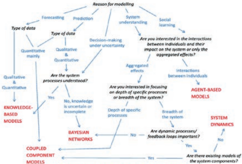
Fig. 1. Decision tree for selecting the most appropriate integrated modelling approach under standard application.
